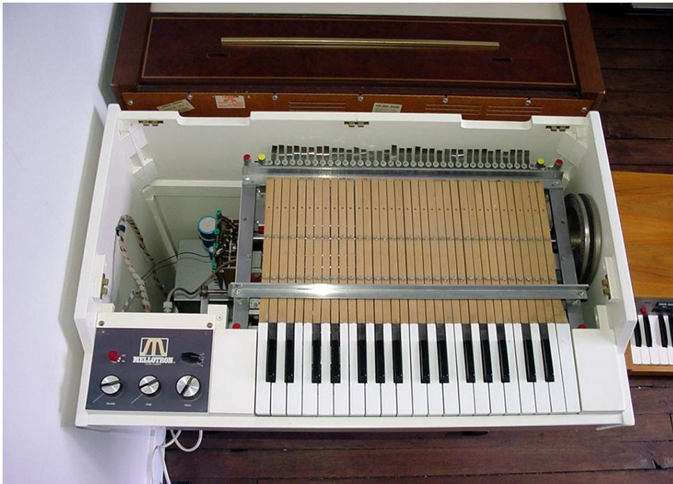
Fig. 2 M400 mellotron, with 35 keys, 35 magnetic tape strips and inner motor mechanism.
