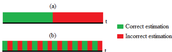
Figure 3.1: Importance of time continuity and grouping of erroneous frames.
