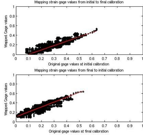
**Figure 3.** Mapping of measured values in similar scenarios for two calibrations: a) Mapping from initial to final calibration; b) Mapping from final to initial calibration.
