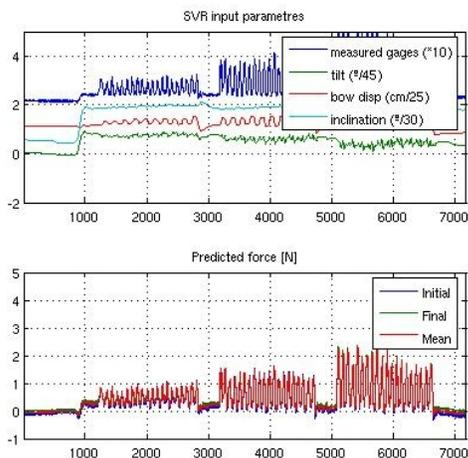
**Figure 4.** Example of measured parameters and predicted forces: a) measured values that will feed the trained SVR models and b) predicted forces by converting the the gage values
