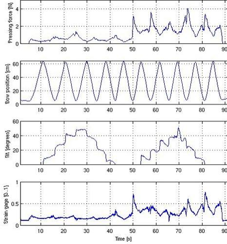
**Figure 2.** Recorded data from calibration: a) Pressing force measured at the load cell [N], b) Bow position [cm], c) Tilt [degrees] and d) Strain gages [0..1].
