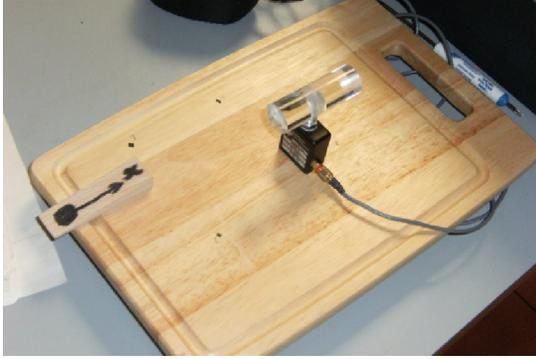
**Figure 1.** Load cell Transducer Techniques MDB-5 with the methacrylate virtual string and wood support.
